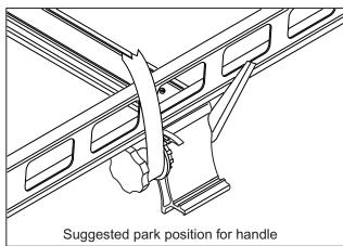
If handle is to be kept on winch shaft, engage as shown to prevent swinging and wear
